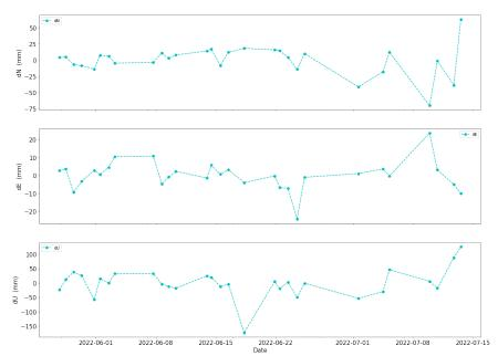
**Figure 4.** Graphs showing position time series for PROION station KRHN (Krini, Aigion). Top panel shows the N-S component, middle panel the E-W component and bottom panel the Up-Down component, respectively.
