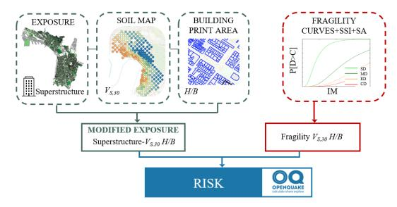
**Figure 1** Methodological framework providing fragility functions including SSI and site amplification expressed in terms of an improved taxonomy. Proposed approach to modify the exposure model to account for SSI and SA through globally available data
