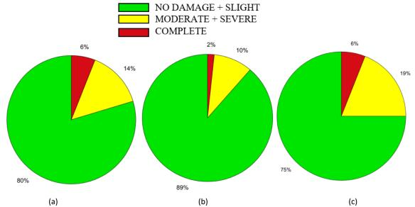
**Figure 2** Aggregated physical damages for most heavily damaged typology during Mw 6.5, 1978 Volvi EQ computed following the approach proposed in this work (a), the literature approach (b), and the actual damage data (c).
