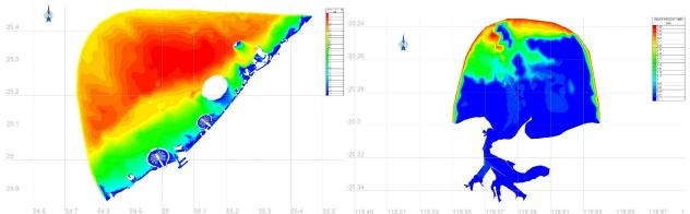
**Figure 2.** Maps of Model A results for significant wave height  $H_s$  (m) in Jebel Ali (left) and Port Headland (right) coastal areas with port approaches during extreme wave conditions,  $H_s = 6m$  and 4m, for north-westerlies and northerlies, respectively.
