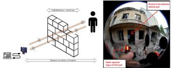
Figure 2. Signs of life detection tool principle of operation (left) and photo from the field trial (right).
