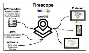
Figure 1. Overview of the architecture of Firescope.
