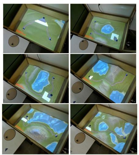
**Figure 2.** Firefighting simulation using the SandMap. Different scenarios result in different, easy to be interpretated visualizations of the fire spread and the optimal pathfinding route.
