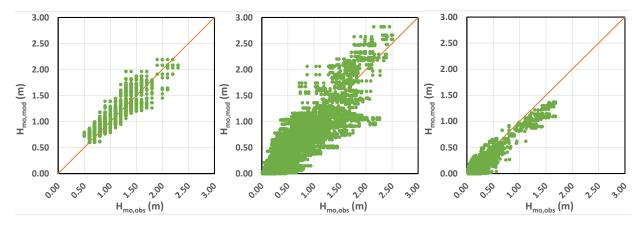
**Figure 1.** Scatter diagrams of comparisons between values of  $H_{mo}$  (m) from Model A simulation outputs (mod) and wave-buoy field data (obs) for the ports of Los Angeles (left), Antwerp (middle), Algeciras (right).
