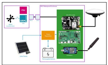
**Figure 2.** The basic elements of the PROION low-cost GNSS system architecture including a component for solar panels for fully autonomous operation.
