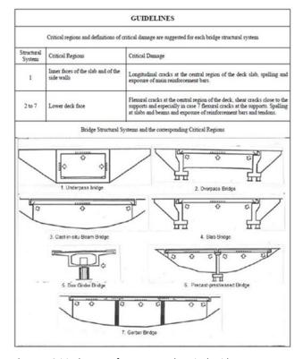
Figure 1 Critical Areas of Damage and Typical Bridge Forms
