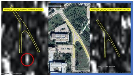
**Figure 3.** SAR amplitude images of the University of Patras Campus showing the location of the corner reflector (red circle). The reflector is oriented at N260°E towards the view direction of the Sentinel-1 ascending orbit.
