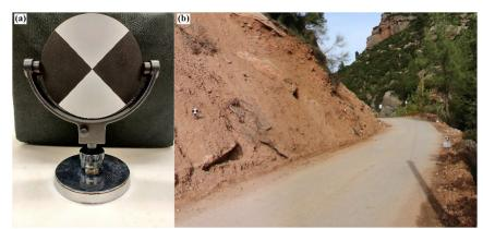
**Figure 2**. (a) 4.5" black and white target for TLS methodology of data aquizition. (b) Distribution of ground control points within the area of interest.
