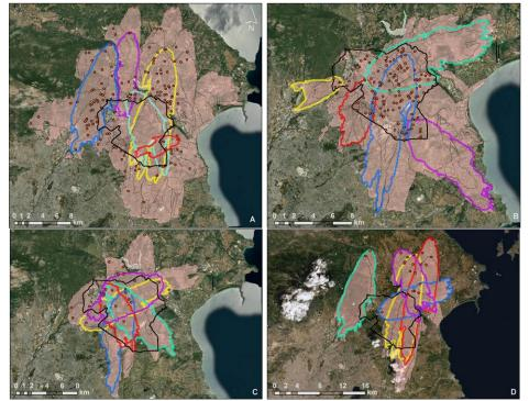
**Figure 2.** Ignition points and simulated fire perimeters: (A) from areas outside Dionysos boundary (B) from areas within Dionysos boundary (C) that may cause the greatest impact on the buildings of Dionysos. (D) The largest simulated fires that entered Dionysos boundary. For a better visual understanding of the results, the five most characteristic perimeters have been colored.
