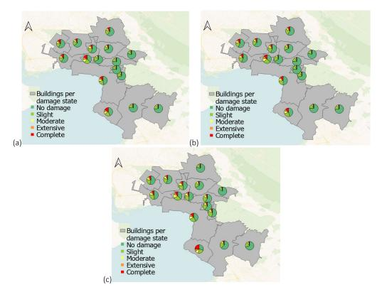
**Figure 3.** Percentages of buildings per damage state for the residential building stock of Thessaloniki per municipality (T=475 years) using for the seismic hazard (a) EAK 2003, (b) current EC8, (c) the proposal for the Greek National Annex of the revised EC8
