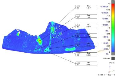
Figure 4. Cloud to cloud comparison between the TLS point clouds, acquired on June 10<sup>th</sup>,2020 and September 25<sup>th</sup>, 2020.
