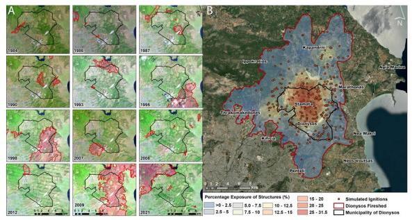
**Figure 1.** (A) Reconstructing the perimeters of the most important wildfires using Landsat satellite images for the period 1984-2021. (B) The fireshed of the Municipality of Dionysos. The color grading shows how many buildings can be potentially affected from future wildfires in each area.
