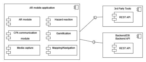
Figure 1. Logical Architecture Diagram of AEOLIAN AR Mobile App.
