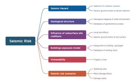
Figure 2. The Methodological framework for seismic risk assessment in Attica Region
