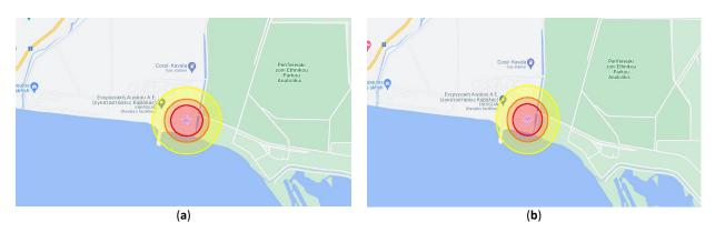
Figure 2. (a) Thermal radiation threat zone for warm season, (b) Thermal radiation threat zone for cold season
