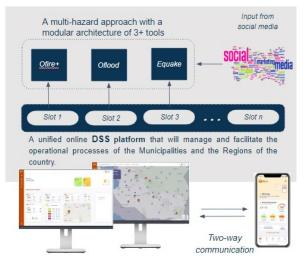
Figure 1. Modular architecture of LocalPro platform
