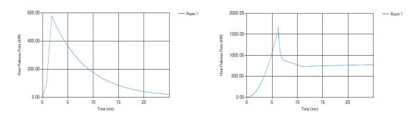
Figure 2. HRR development over time for the 1st scenario (left) and 2<sup>nd</sup> scenario (right)
