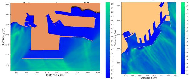
**Figure 3.** Maps of Model B, very fine resolution results, for pseudo-spectral wave height H (m) in Algeciras (left) and Buenos Aires (right) ports during high wave conditions, H≈2m, for easterly to south-easterly winds, respectively.
