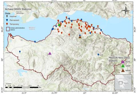
**Figure 1.** Relief map of Achaia Prefecture (western Greece) showing PROION sites (solid triangles) and other geodetic installations mostly belonging to the CRL Near Fault Observatory (https://nfo.crlab.eu/).
