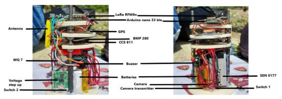
Figure 2. Structural design of the FireSat
