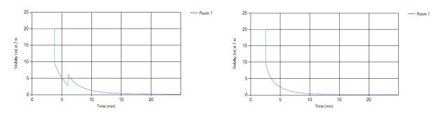
Figure 3. Visibility development over time for the 1st scenario (left) and 2<sup>nd</sup> scenario (right)
