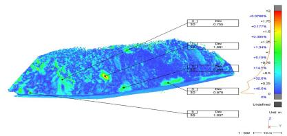
Figure 3. Cloud to cloud comparison between the UAV point clouds, acquired on June 10th,2020 and September 25th, 2020.
