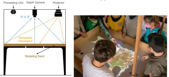
Figure 1. The SenseLab's SandMap architecture (left) and its demonstration (right).
