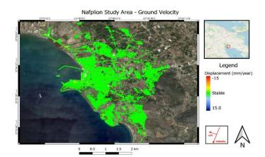
The interferometric process successfully reflects the trends of surface deformation of each area. The territorial background of the city of Nafplio shows stability at a depth of 8 years while also areas with intense impending soil subsidence are identified. In particular, the impending deformations in the north wing of the old city are quite rapid, reaching up to half a meter every two years, while subsidence is also found in the eastern zones.
