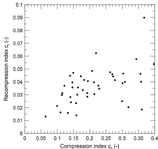
Figure 14. Dependency between  $c_c$  and  $c_r$ .
