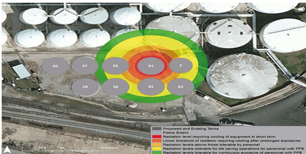
Figure 4. Thermal radiation zones in refinery fuel storage tanks in case of fire (D'Amico 2015)
