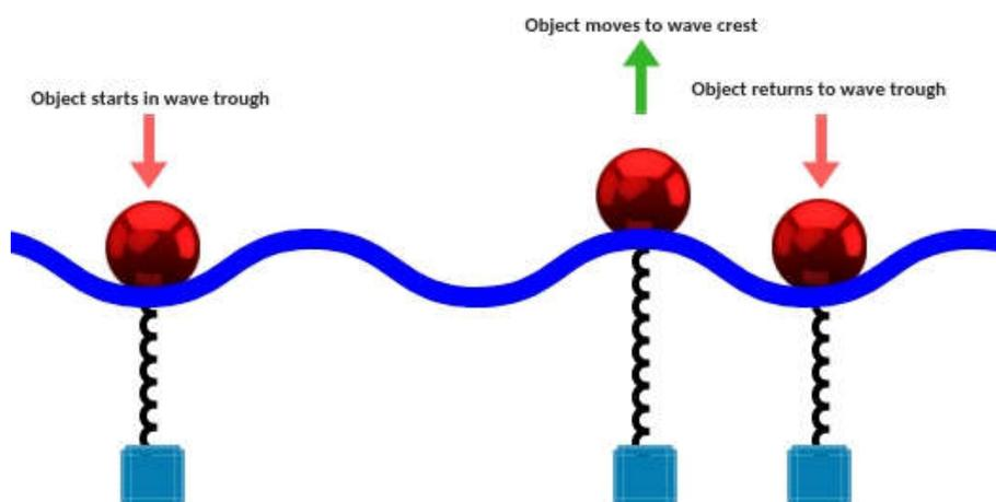
Figure 1. Concept of Wave Power Generation
