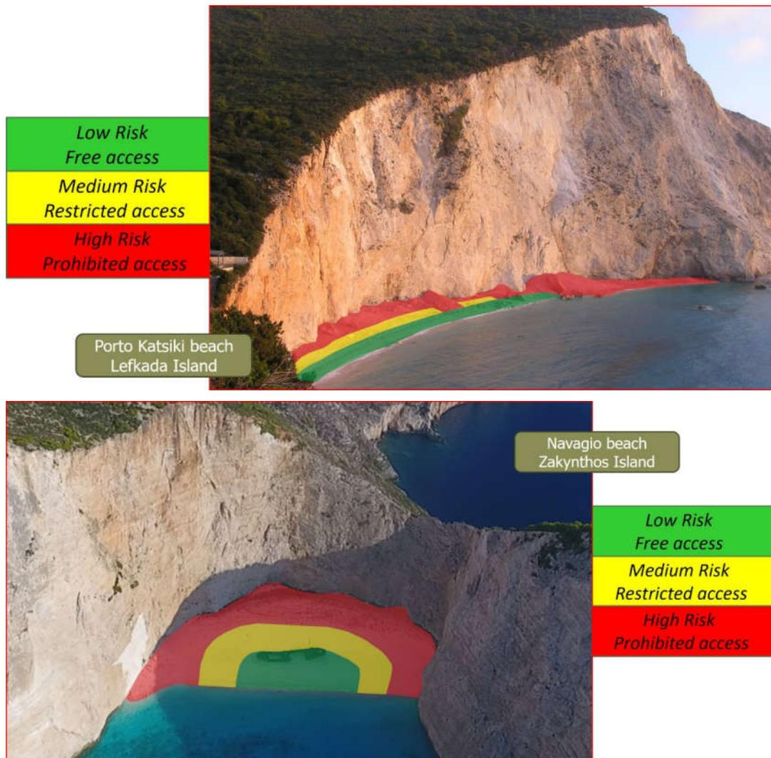
**Figure 4:** Application of the beach zonation for mitigation of landslide risk and responsible tourism development in Porto Katsiki (up) and Navagio (down) beaches in the western part of Lefkada and Zakynthos respectively.
