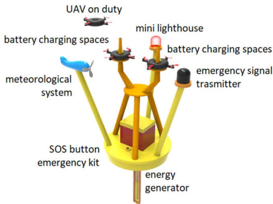
Figure 3. Part description of the ANASA Unit (design is still under development)
