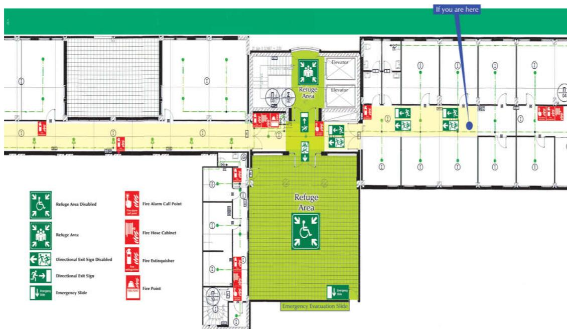
Figure 2. Part of a “Fire Escape Plan” based on the last updated International Standard, ISO 23601:2009 (Safety identification -- Escape and evacuation plan signs)- Incorporation of the new egress symbols, especially designed for disabled people
