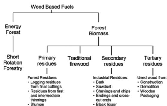
Fig. 3. Wood based fuels - classification (Röser et al., 2008).
