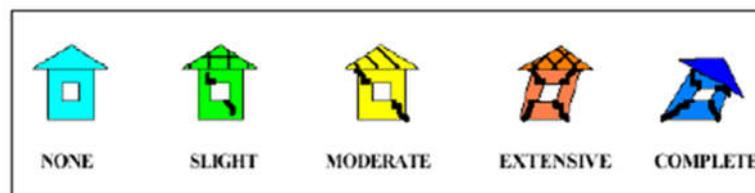
Figure 3: Damage Levels (FEMA, 2001)
