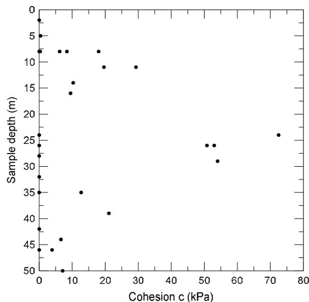
Figure 13. Variation of cohesion with depth.
