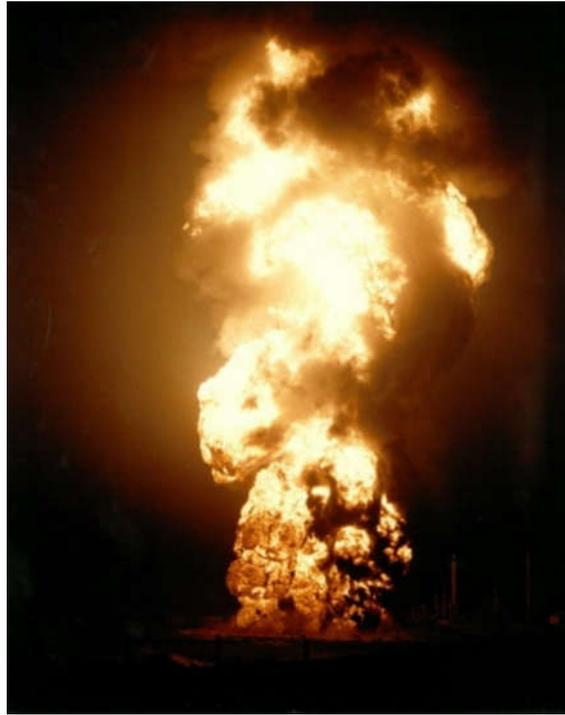
Figure 2. Boilover in a crude oil tank at the Milford Haven accident (Courtesy of Mid and West Wales Fire and Rescue Service from Dyfed County Fire Brigade, 1983)
