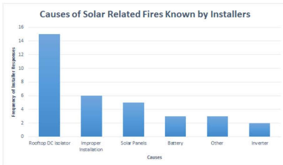
Figure 7. Causes of solar-related fires reported by installers in Australia (Chiaramonte et al 2016)
