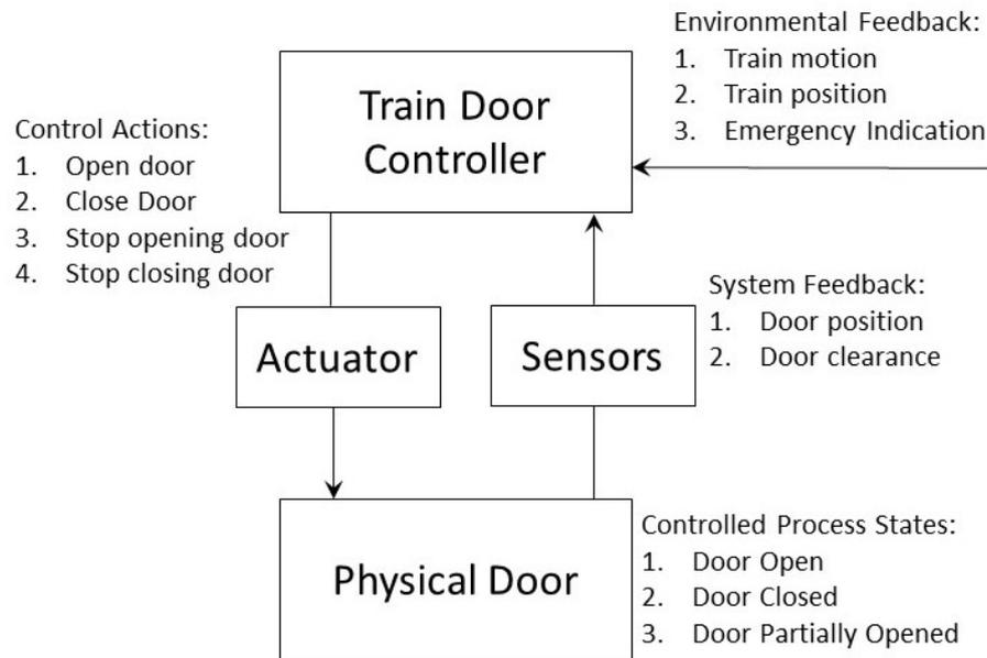
**Figure 4:** Train Door System Safety Control Structure
