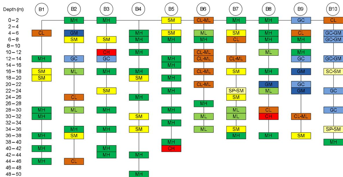
Figure 11. Classification of spoil material (according to USCS) along the longitudinal axis of the spoil heap.
