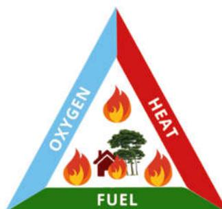
Fig. 1. The Fire Triangle. The forest fires are results of combustion. A chemical reaction which combines three factors. The Oxygen, the Heat and the Fuel. The sustainable Forest Biomass extraction for energy utilization would reduce the forest fire risk by reducing the fuel source in a viable and ecological way.
