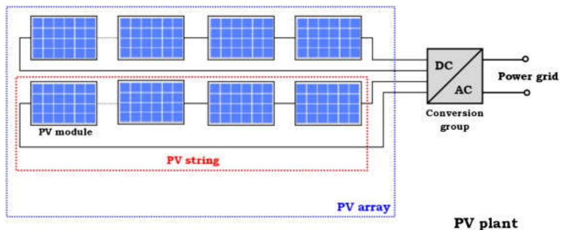
Figure 2: Configuration of PV systems (La Manna et al 2014)
