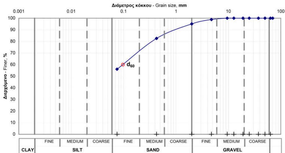
Figure 12. Indicative grain size distribution curve on a spoil heap sample.
