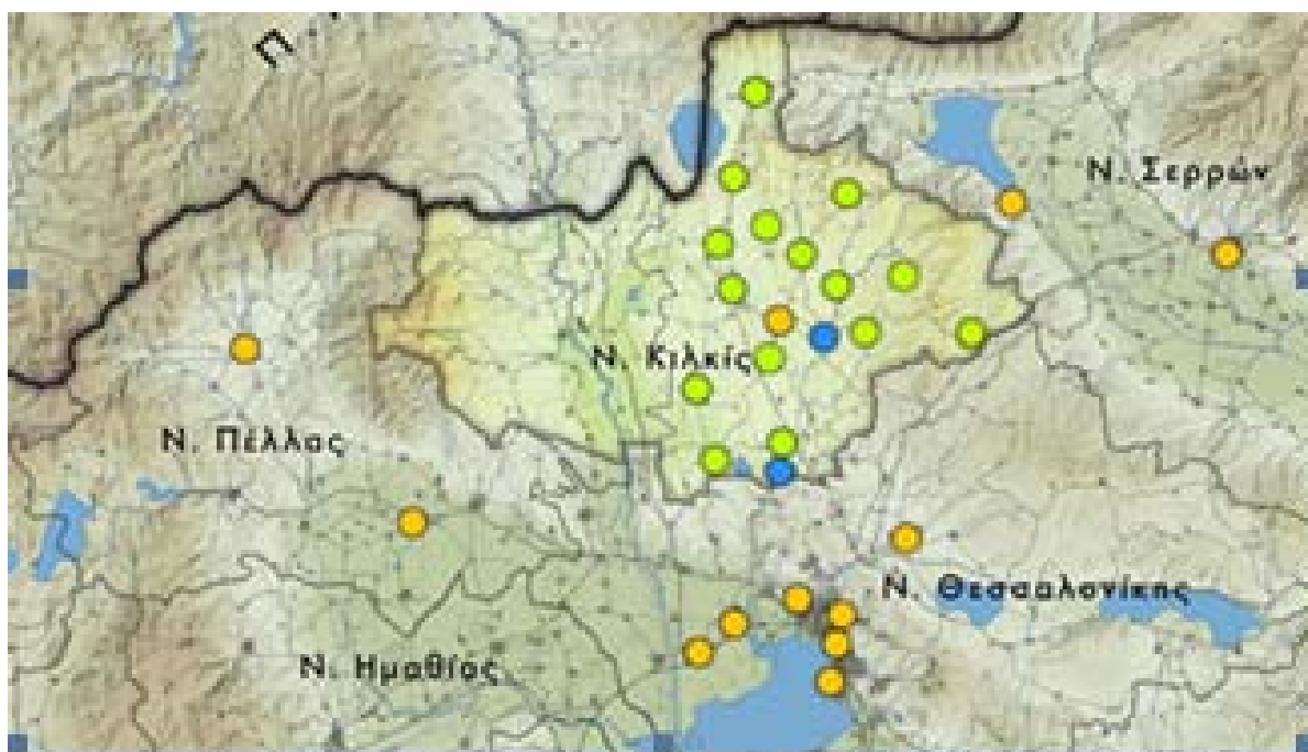
Figure 1. Map of proposed new meteorological stations (green dots) and level meters in Gallikos River (blue dots). The orange dots indicate the positions of the existing stations of the National Observatory of Athens.
