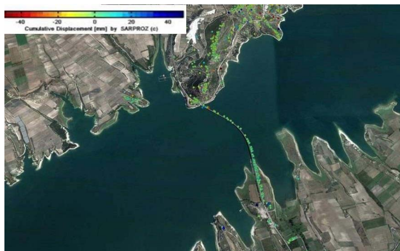
Figure 2. PSI deformation map (Non-Linear deformation, cumulative in mm)
